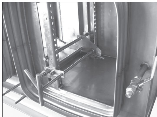
Scan Probe Assembly with Scanning Wand and Ball Valve Shutoff
