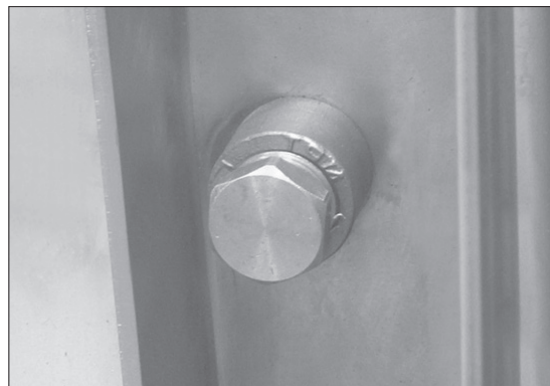
Static Pressure Taps are 1/4-inch Stainless Steel Half-Coupling with Brass Hex Plugs
